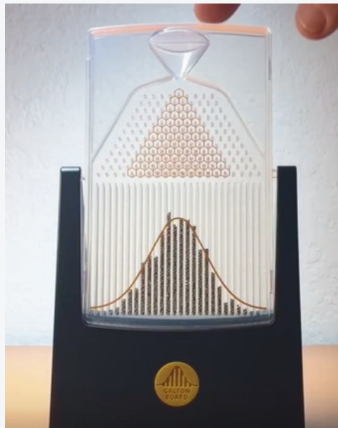
Figure 27: The Galton Board, linking Pascal's Triangle to the normal distribution
