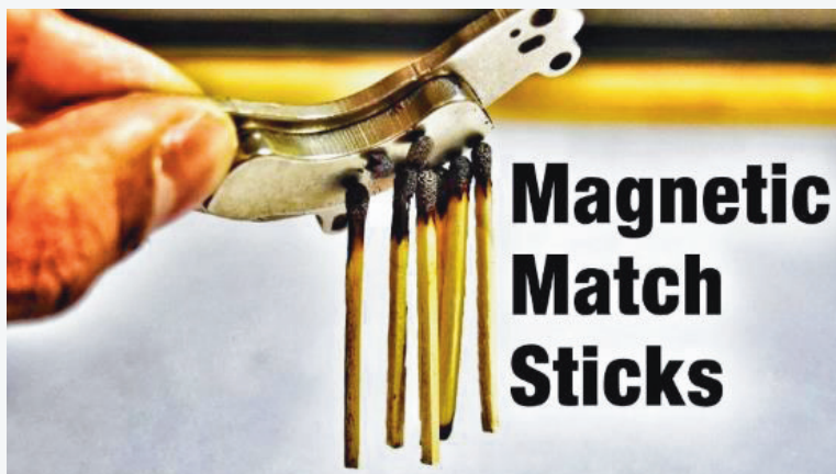
Figure 26: Matches become magnetic after burning, a discrepant event for chemistry
