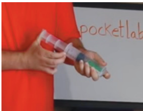
Figure 53: Measuring Boyle's Law using the PocketLab and a sealed plastic bag or a syringe
