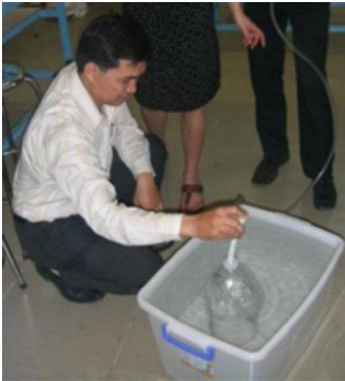
Figure 7: functioning of the low-cost spirometer
