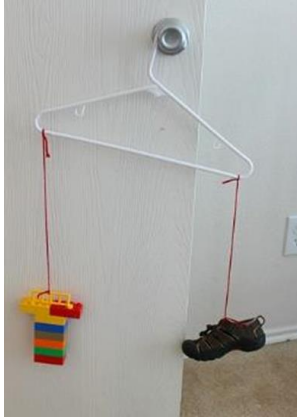
Picture 70 A self-made scale from a clothes hanger. Which is heavier, the shoe or the toy?
